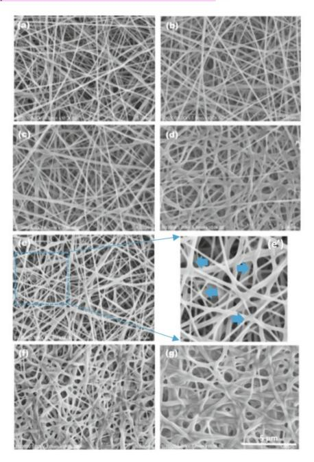
**Fig. 1** SEM images of the electrospun nanofiber membranes of neat PVA (a), AVF-10/PVA (b), AVF-20/PVA (c), AVF-30/PVA (d), AVE-1/AVF-30/PVA (e), a magnified image of a square area marked in Fig. 1e (e'), AVE-3/AVF-30/PVA (f) and AVE-5/AVF-30/PVA (g)
