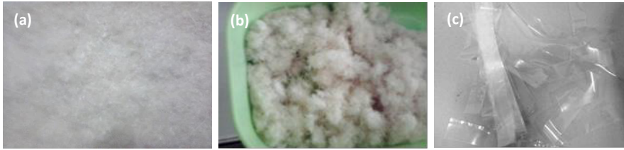
Figure 1: Photographs of short sisal fibers (a) before, (b) after alkalization and (c) PP sheets used at the polymer matrix
