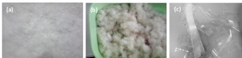
Figure 1: Photographs of short sisal fibers (a) before, (b) after alkalization and (c) PP sheets used at the polymer matrix
