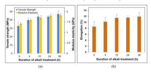
FIGURE 3. Tensile strength and modulus (a) and elongation (b) versus duration of alkali treatment.
