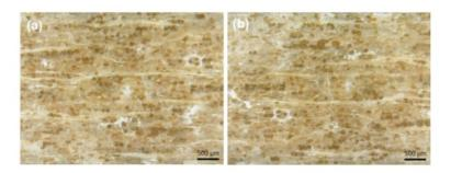
FIGURE 5. Optical micrographs of kenaf fibers dispersion in the PP matrix obtained from the specimen with untreated (a) and treated fibers for 4 h (b).
