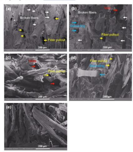
FIGURE 4. SEM images of tensile fracture surface obtained from the composite specimens with different alkali treatment durations of kenaf fibers. (a) Untreated, (b) 4 h, (c) 10 h, (d) 24 h, and (e) 36 h.
