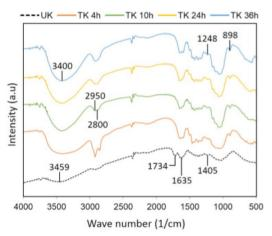
FIGURE 2. FTIR spectra of untreated kenaf (UK) and alkali treated kenaf (TK) fibers.
