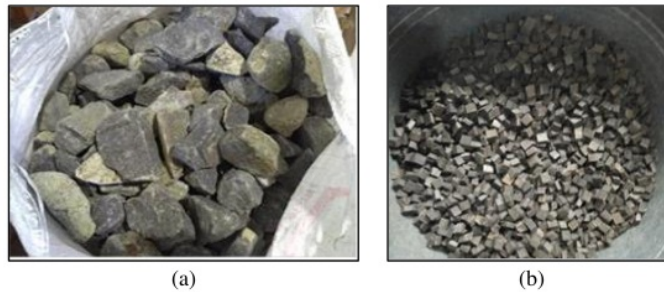
Fig. 1 - (a) Ballast materials; (b) Scrap rubber.
