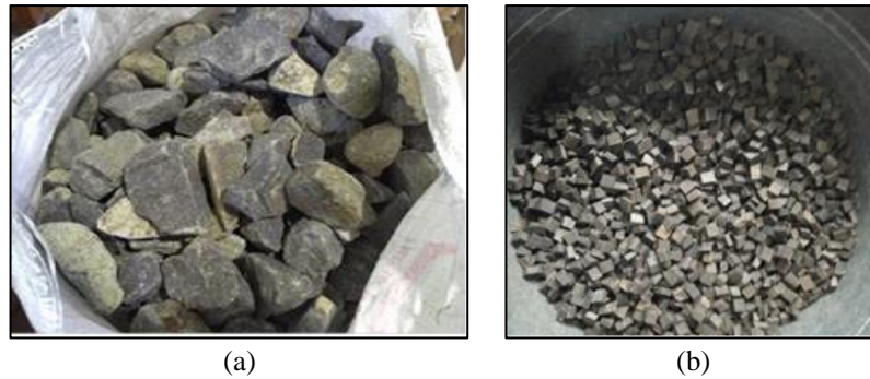
Fig. 1 - (a) Ballast materials; (b) Scrap rubber.
