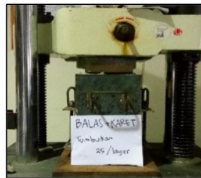
Fig. 3 - compressive test process with UTM tools.
