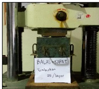
Fig. 3 - compressive test process with UTM tools.
