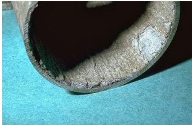
Gambar 2.6 Korosi Intregranular (Mechanicalengineering, 2014)
