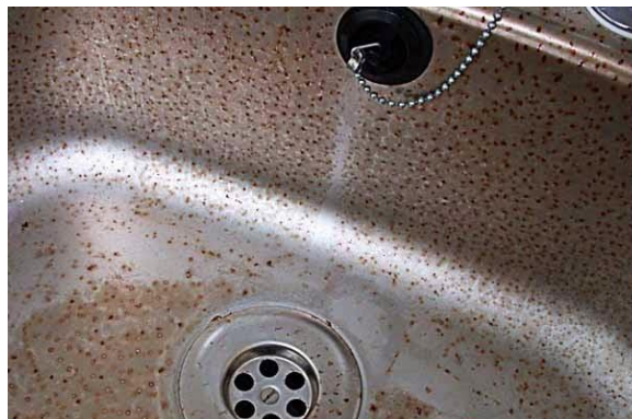
Gambar 2.5 Korosi Sumuran (Mechanicalengineering, 2014)
