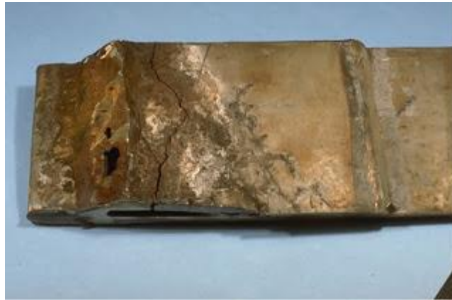
Gambar 2.7 Korosi Retak Tegangan (Mechanicalengineering, 2014)
