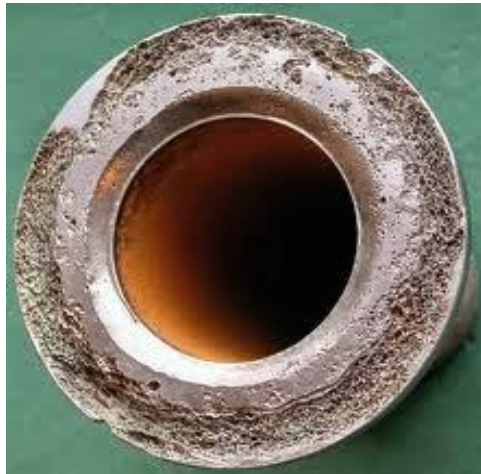
Gambar 2.4 Korosi Celah (Mechanicalengineering, 2014)
