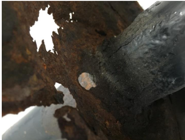
Gambar 2.3 Korosi Selektif (Mechanicalengineering, 2014)
