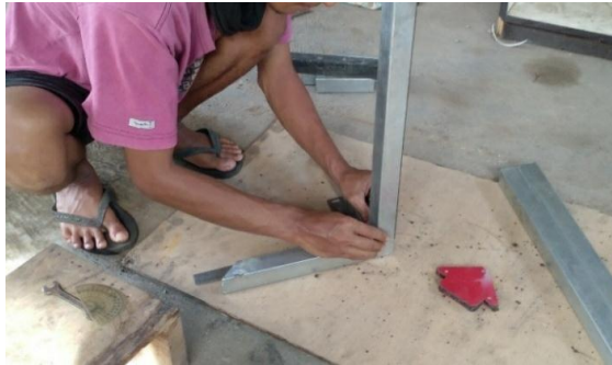
Gambar 3.2. Proses Setup Tanpa Menggunakan Three Axis Fixture Vise
