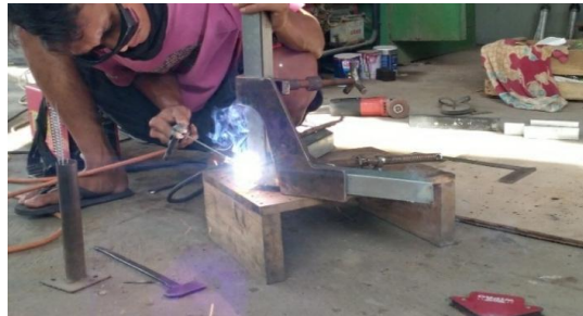
Gambar 3.3. Proses Pengelasan Menggunakan Three Axis Fixture Vise
