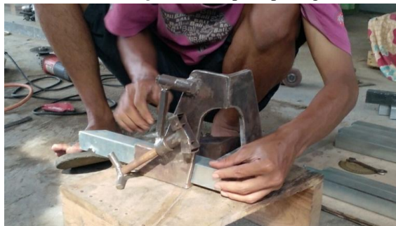
Gambar 3.1. Proses Setup Menggunakan Three Axis Fixture Vise
