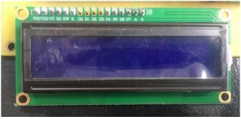
Gambar 2.29 Liquid Crystal Display16x2
