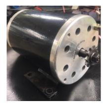
Gambar 2.7 Motor DC 1000 Watt 48 Volt
