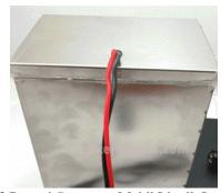
Gambar 2.3 Baterai *Prototype* Mobil Listrik Jenis Lithium Ion
