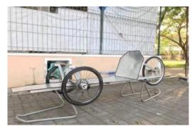
Gambar 2.1 Prototype Mobil Listrik
