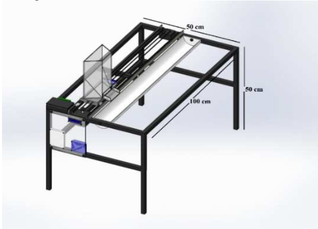
Fig. 3. Design of the Feeding Automation Tool
