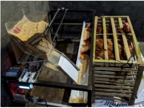
Fig. 6. Overall Feeder Automation Equipment for Laying Hens
