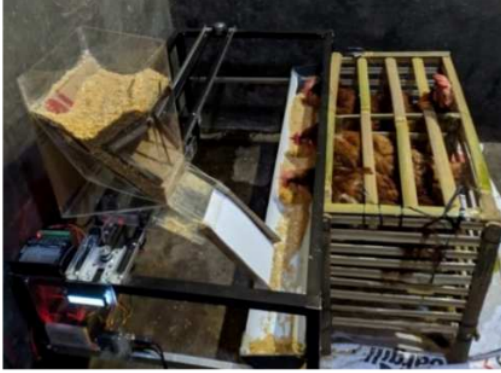
Fig. 6. Overall Feeder Automation Equipment for Laying Hens
