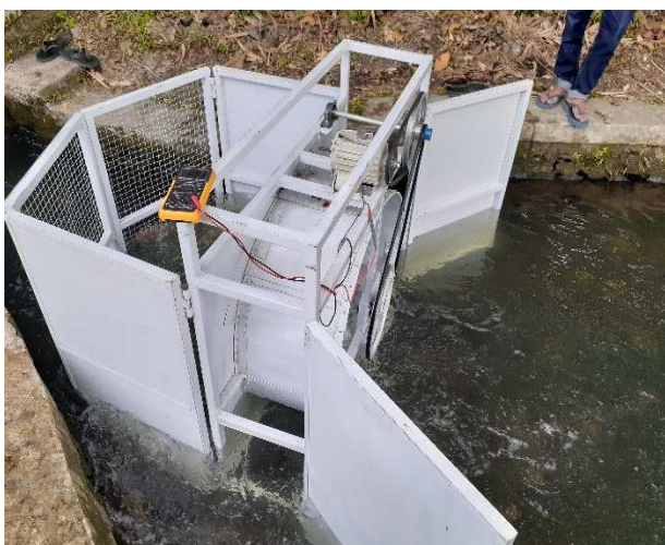
Fig. 2. Testing of a small hybrid renewable power plant in an irrigation canal
