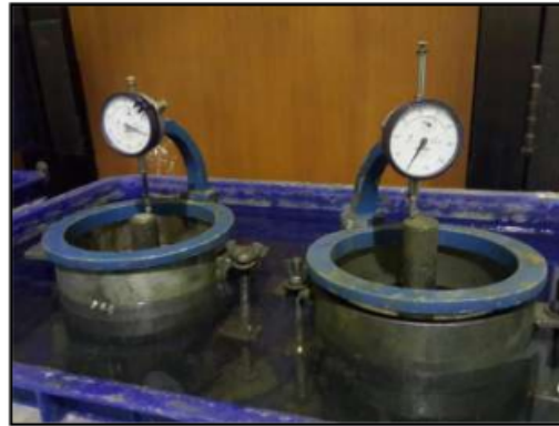
Fig. 3. The immersion of specimens for four days before CBR penetration test
