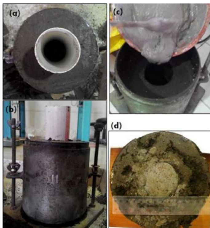
Fig. 2. Specimen preparation (a)-(b) soil compaction in CBR cylinder and column hole, (c) pouring SiCC paste in the hole, (d) SiCC column after hardening
