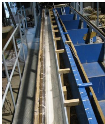
Photo 1 The flume test channel and the flow direction is to bottom side
