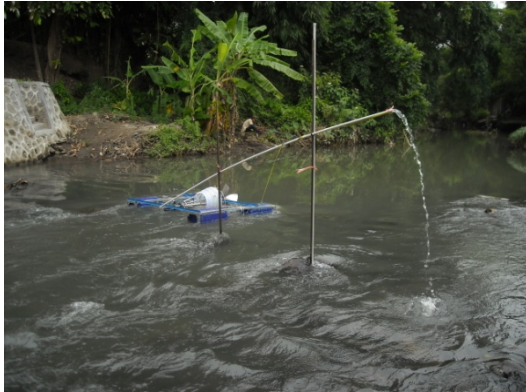
Gambar 1. Penelitian Sling Pump di Sungai Bedog
