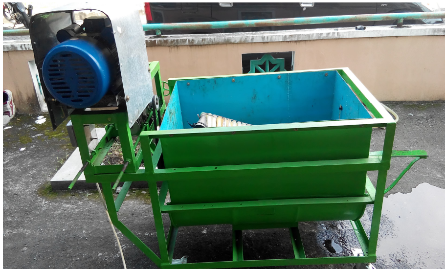
Gambar 3.1. Sling pump skala laboratorium
