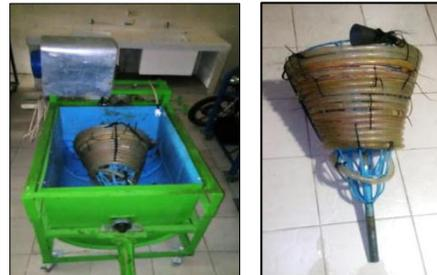
Gambar 7. Prototype *sling pump*
