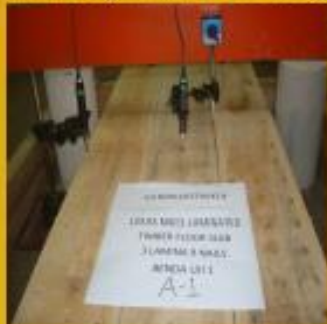
CNLT floor under vibration test
