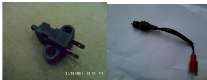
Gambar 2.15. Switch lampu rem handel kiri Yamaha Mio (otosportmaniak, 2016)
