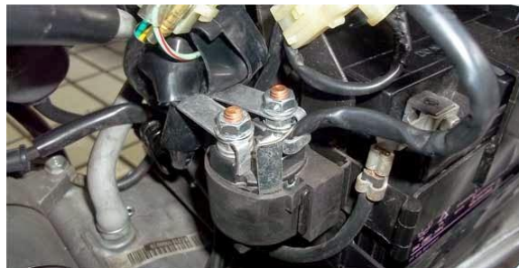
Gambar 2.31. Relay starter (motor-hargaku, 2015)
