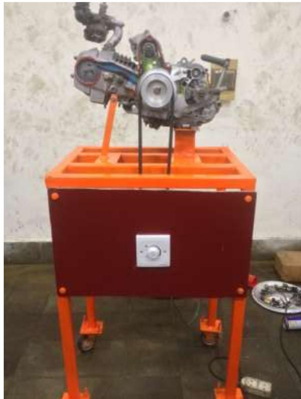
Gambar 4.1. *Stand Engine Cutting*
