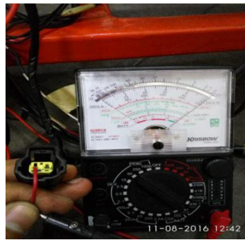
Gambar 4.17. Memeriksa Sensor Suhu Mesin ( Engine Temperature Sensor )
