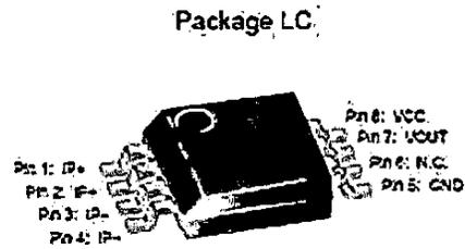
Pin 6 and 7 are internally connected in shipping product. For compatibility with future devices, leave pin 6 floating.
