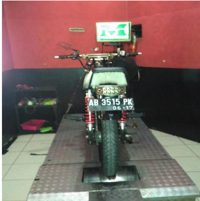
Gambar 2.8 Mesin *dynamometer test*
