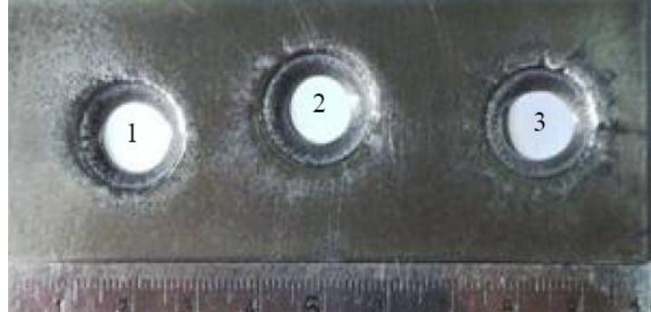
Gambar 2.4 Prinsip contoh hasil drilling ECM hardened tool steel SKD 11 dimensi 100 x 40 x 4.5 mm (Suhardjono, 2014)
