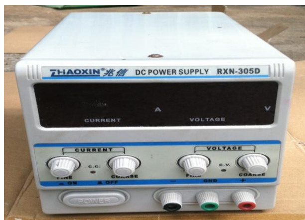
Gambar 3.2 DC Power Supply
