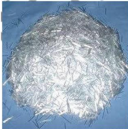
Gambar 2.13. Serat gelas chopped strand (Sudarman, 2014).
