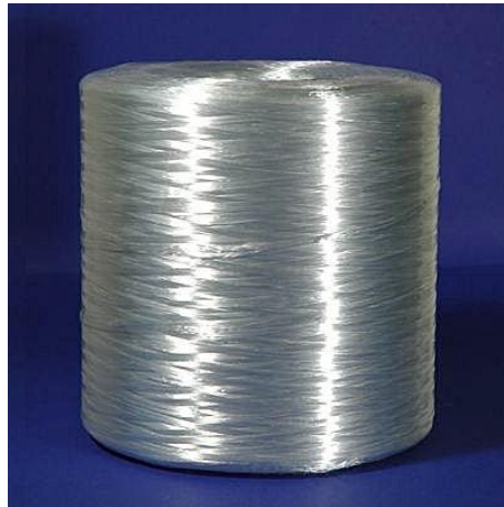
Gambar 2.11. Serat gelas roving (Sudarman, 2014).
