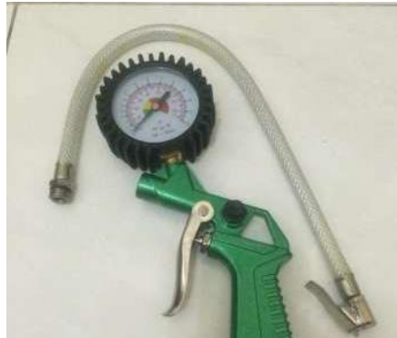
Gambar 3.13. Tire Pressure Meter
