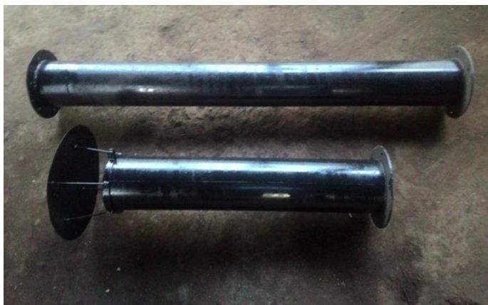
Gambar 4.27 Cerobong asap incinerator
