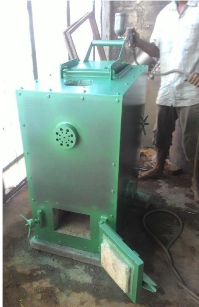
Gambar 4.29 Proses pengecatan incinerator
