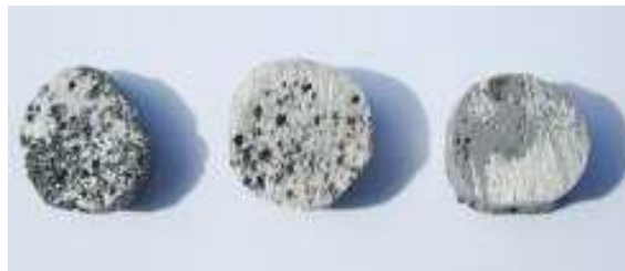
Gambar 2.1. Produk aluminum Foam (a. 4%Mg; b. 6%Mg; c. 8%Mg) (Agustian, 2012).
