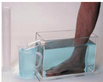
Gambar 2. 1. Baseline Volumemeter Measuring Device Foot , 5x13x6 inches Sumber: Brodovicz, 2009. reproduced with permission from WisdomKing.com viwed 2 Maret 2015, www.wisdomking.com
