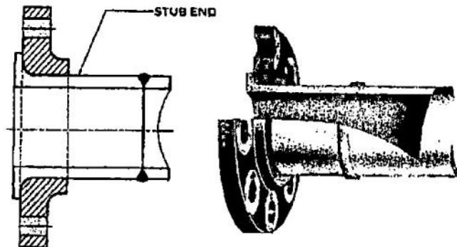
**Gambar 3.6. Flange Lap Joint**
