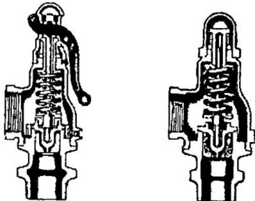
**Gambar 3.13. Safety Valve/ Relief Valve**
