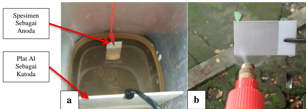
Gambar 3.35 (a). Proses Anodic Oxidation , (b). Proses Rinsing
