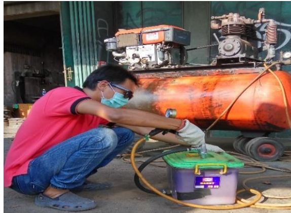
Gambar 3.21. Proses perlakuan shot peening
