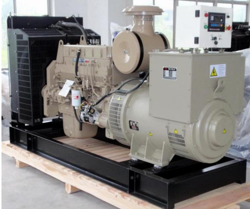
Gambar 2.4. Genset Tipe Open Merk Cummins (Sumber: http://gudanggenset.com )
