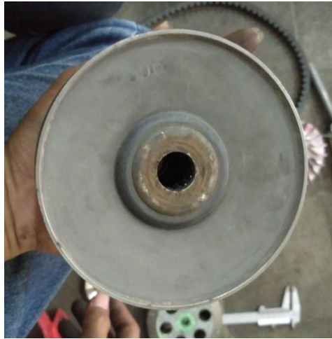
Gambar 4.9. memeriksa secondary fixed sheave
