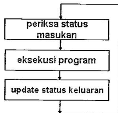
Gambar 2.4. Proses Scanning Program PLC
