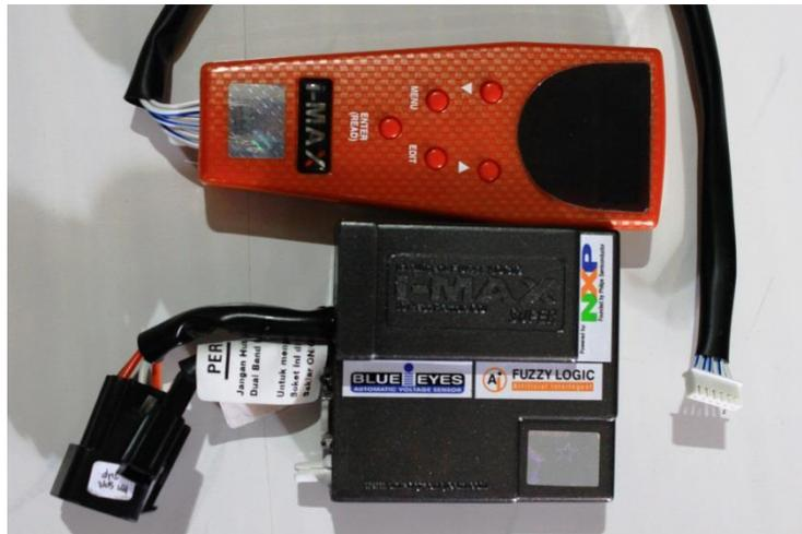
**Gambar 3.1.** CDI BRT I-Max 24 step *programmer*.
