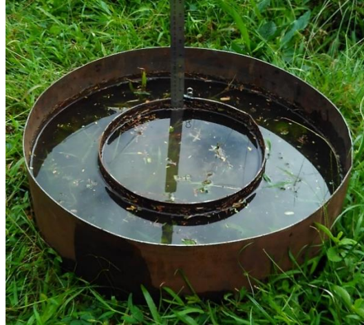
Gambar 4.3 Alat double ring infiltrometer
