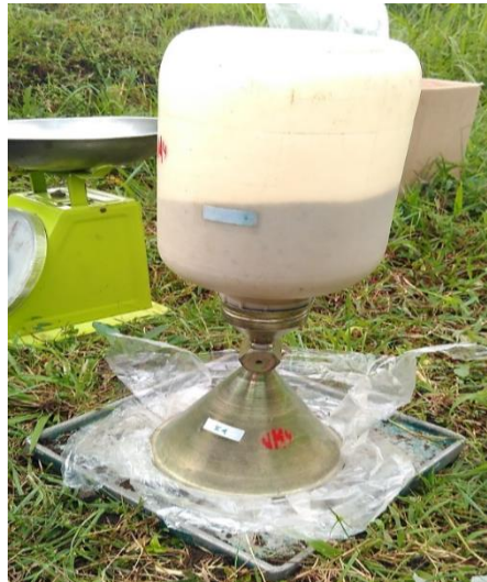
Gambar 4.5 Alat kerucut pasir ( sand cone )
