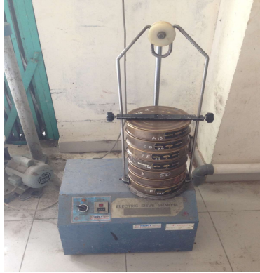
Gambar 4.10 Electric sieve shaker machine
