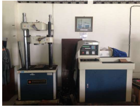
Gambar 4.9 Universal testing machine
