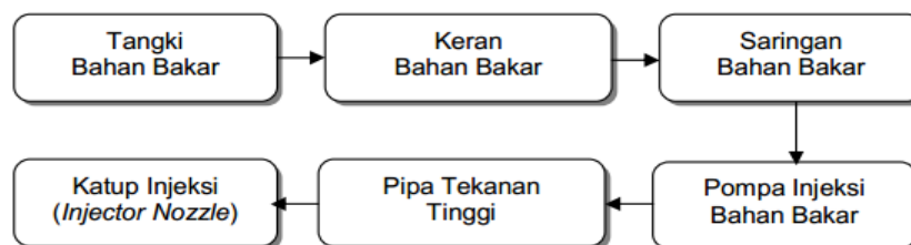
Gambar 2.7. Diagram aliran system bahan bakar
