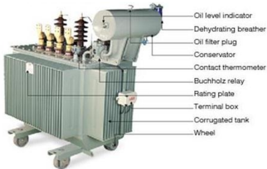
Gambar 2.2 Bagian-bagian Transformator Daya
