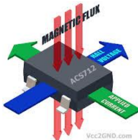
Gambar 2.8. Sensor Arus Magnetik Sumber: http://www.vcc2gnd.com/sku/ACS712-5
