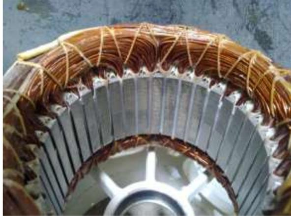
**Gambar 2.7** Gambar Stator Generator Sinkron
