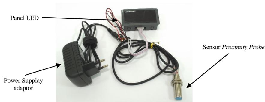
Gambar 3. 7 *Tachometer Proximity Probe*
