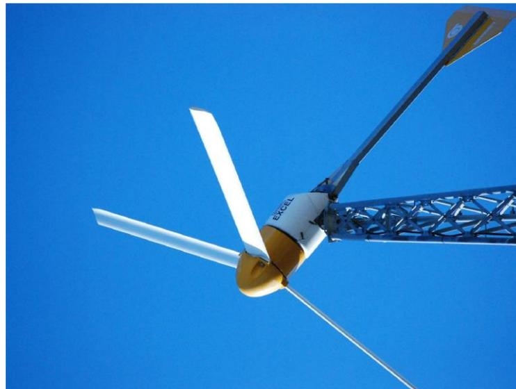
**Gambar 4.15** Turbin Angin BWC EXEL-S 10kW**Table 4.8** Spesifikasi Turbin Angin BWC EXEL-S 10kW
