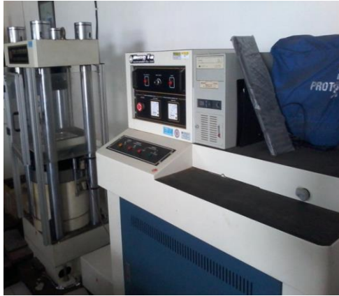
Gambar 4.19 Alat uji tekan concrete compression tester machine merk “Hungta”
