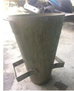
Gambar 4.5 Kerucut Abrams
