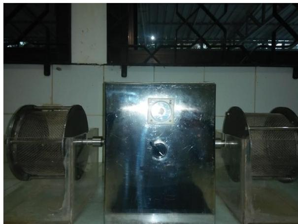
Gambar 3.5 Alat Uji *Slake Durability*
