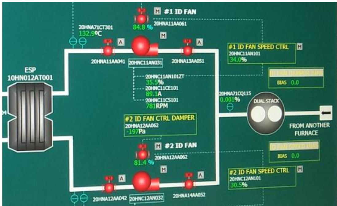
**Gambar 4.4** Digital Monitoring mekanisme kerja *flue gas system* PLTU Sebalang di *Control Room*
