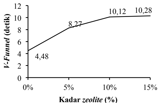
Gambar 3 Hubungan hasil uji v-funnel dan kadar zeolite
