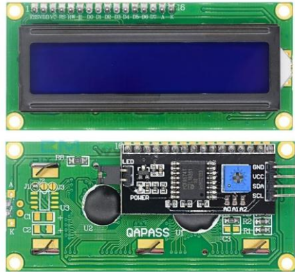
Gambar 2. 7 LCD I 2 C ( Inter Integrated Circuit )[21]
