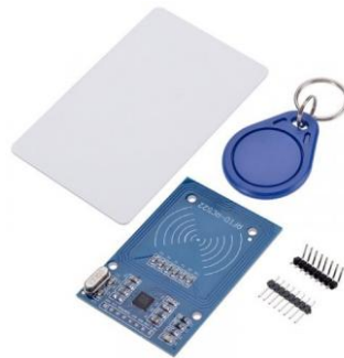
Gambar 2. 3 RFID ( Radio Frequency Identification )[9]
